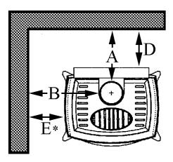
\* Note: E and F dimensions are measured to side of stove below the projection of outer top.
